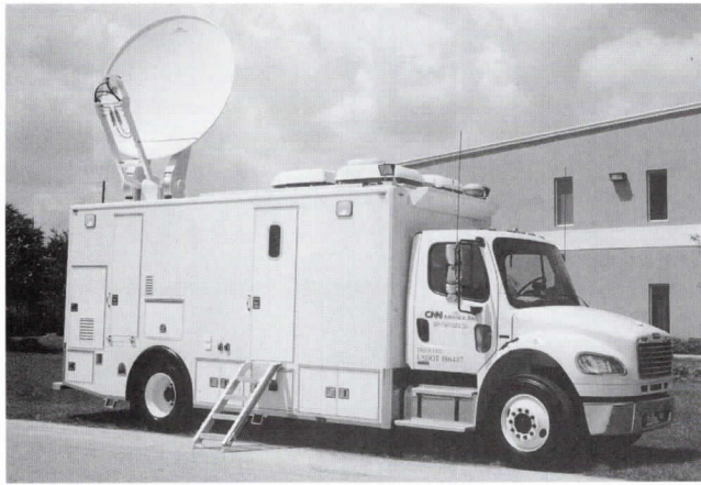
FIGURE 5.17-8 SNG uplink vehicle. (Courtesy of Frontline Communications.)
