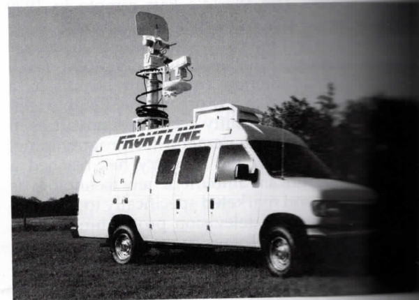
FIGURE 5.17-3 Typical ENG microwave vehicle. (Courtesy of Frontline Communications.)
