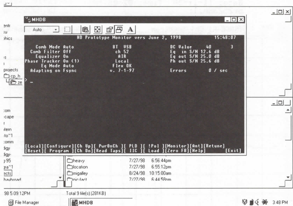
Figure 13.32 Software program that indicates the DSP efforts required in a test receiver to ensure proper decoding of the received DTV signal.
