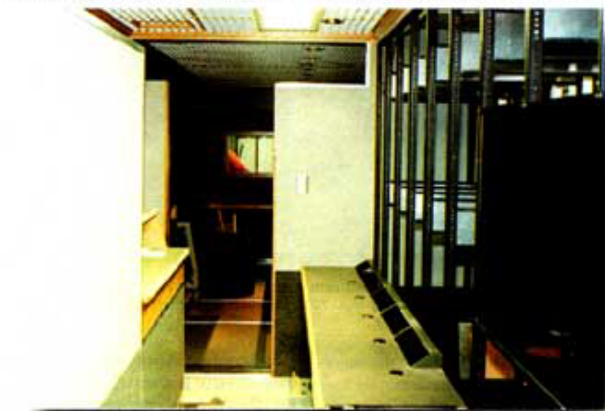
The videotape and control area contain nine racks. The first five racks, shown above, contain five HDW-500 recorders and associated monitors. The next four racks provide video control for up to 16 cameras. Note the large black box on the right. It is used to house one of two HDM-20E1U high-definition monitors.
